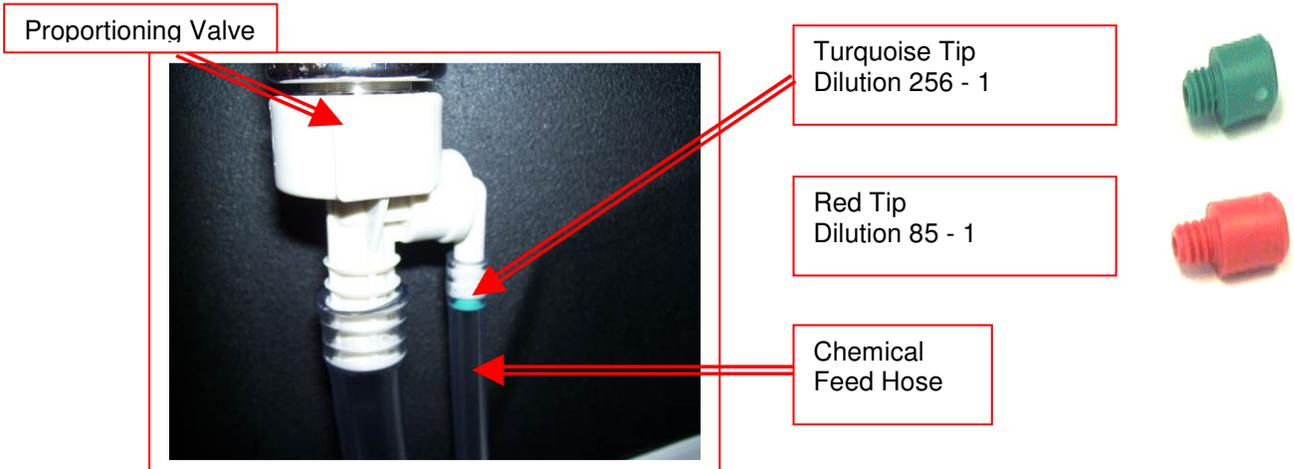
**Metering Tip Kit (Hydro-Force Item# PDE001)** contains 14 different colored metering tips, allowing dilution rates from 11:1 up to 427:1. Refer to the chart below to select the tip that meets the dilution rate for your chemical application.
