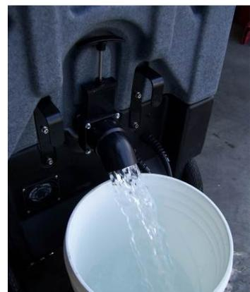
Drain water from Recovery Tank
