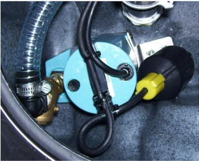
Connect the Female Garden Hose Fitting end of the Pump-out Hose to the outlet fitting on the back of the recovery tank. Place the other end of the pump-out hose in a sanitary drain.
